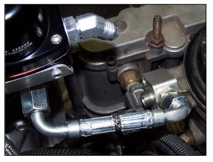
56. If you are using an electric "in-cab" fuel pressure gauge, install the sending unit in the front gauge port
