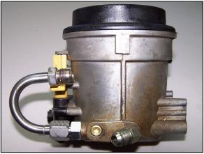
30. Remove the allen head plug from the port to the left of where the pipe plug was installed and replace it with the 04MB-06M1 o-ring fitting included in the kit
