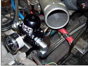
brass colored nut behind the straight hose end to keep the hose from twisting while tightening.
